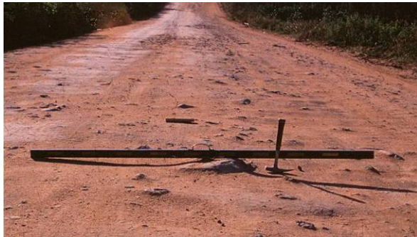
Figure 88. Photo. Estimating gravel loss from stone protrusion.
