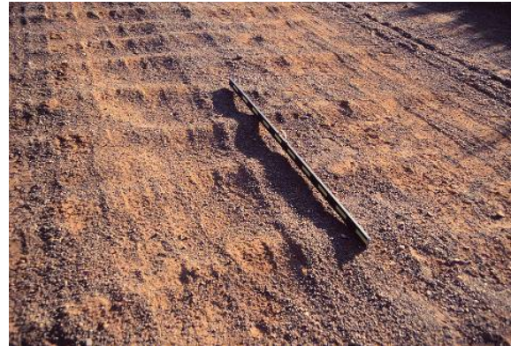
Figure 58. Photo. Poor gravel selection for treated road.
